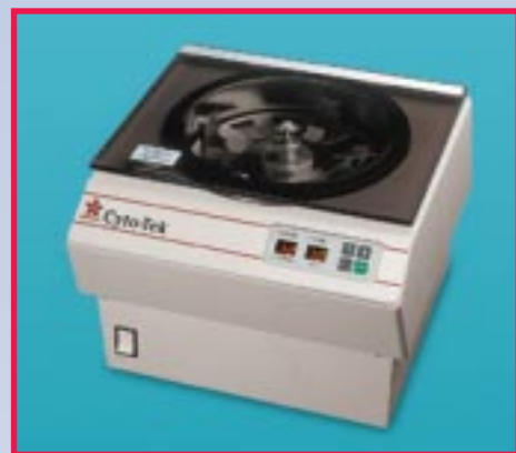
Fig. 3. A cytocentrifuge (like the Sakura Cyto-Tek®) is used to concentrate cells from body fluids when preparing IHC control samples.
